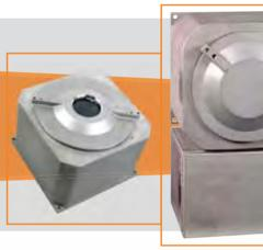
TNCD enclosures, Ex d/de made of stainless steel are designed to meet the requirements for Ex d IIC equipment in harsh environments on- and offshore. TNCD can be delivered as Ex d direct entry or as an Ex de combination for indirect entry.
