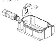
Push the earthing plate (4) for metal cable entries in between the rib and the inside wall of the enclosure. The earthing plate is secured in place when the cable entry is screwed in.
